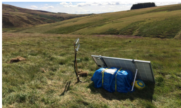
Underline differential magnetometer system in-situ at Whiteadder, Scottish Borders
